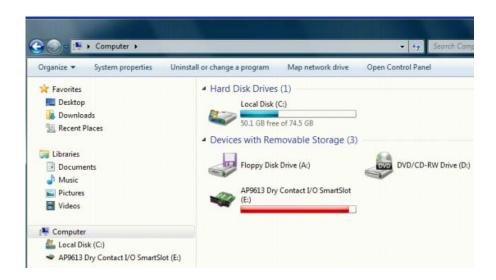
To run the Utility, launch the runme.hta file located in the root of the drive. For information on using the Configuration Utility user interface, refer to its online help.
